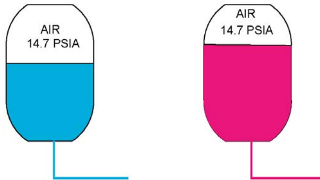
Figure 2: A closed tank with no bladder has free space when the hydronic hot water system is cold. As the temperature within the system rises, the water expands into the free space within the tank.
