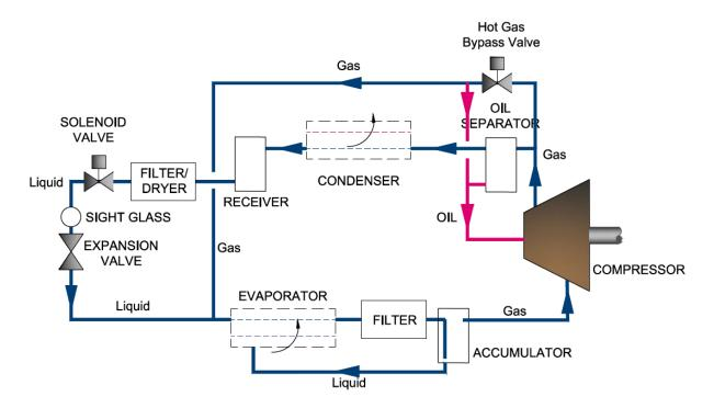
The correct answer is most nearly, (B) A hot gas bypass can be placed between the compressor discharge and the evaporator to create an artificial load.
