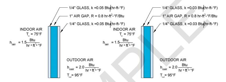
You need to find the overall heat transfer coefficient, U. But it is easier to find the overall heat transfer coefficient by first converting all the heat transfer coefficients to R-values.
