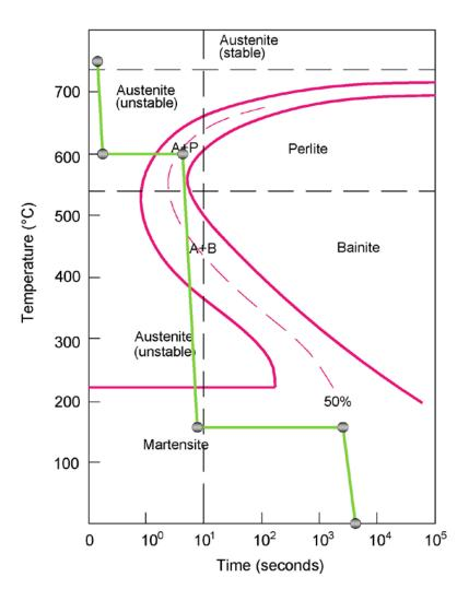
The first two steps will cause more than half of the steel to turn to perlite. The remaining will turn to martensite in the final steps.
