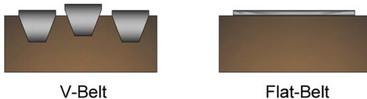
Figure 21: A v-belt has grooves that reduce slippage. A flat belt on a pulley is also shown for comparison.
