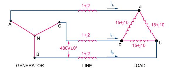
In order to complete this problem you must first convert the delta load to an equivalent wye load. This will help to make a simpler circuit for solving for the line current, since the line current is equal to the phase current. The conversion for delta to wye impedances is to divide the delta impedance by 3.
