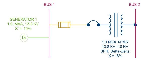
Since Bus 2 is the desired fault location, assume a base of 1 MVA and 1 KV.
