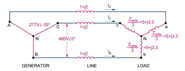
Now the drop along this phase includes the line impedance and the load impedance. With this simple circuit you now have the impedance and voltage and can therefore solve for the current.
