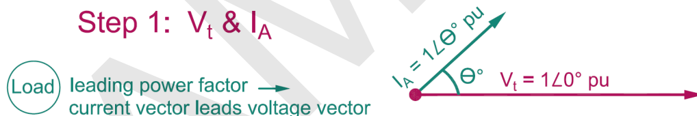
Figure 21: Step 1 - Assign your voltage as having a 0 degree reference point and the armature current leads the voltage phasor by the power factor angle.
